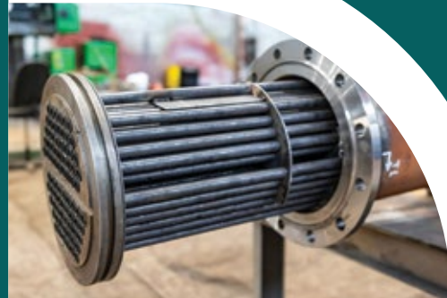
Heat Exchanger Repair
